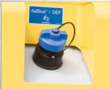
Diesel Exhaust Fluid (DEF) tank
