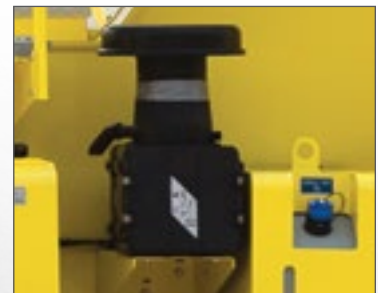
Tier 4 Final integrated pre-cleaner and air filter
