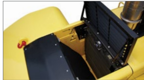
Hinged cover enables easy serviceability access to radiator cooler
