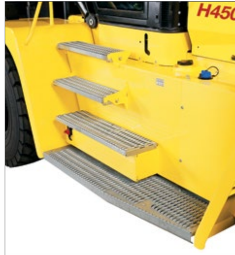
Broad running boards
