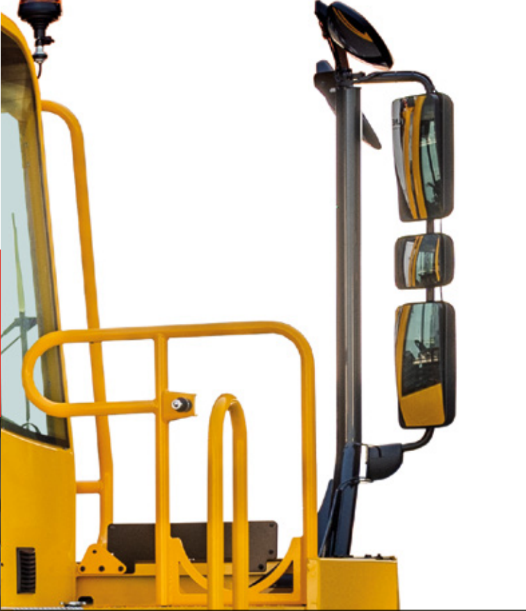
Improved mirror mount. Standard and optional mirrors.
