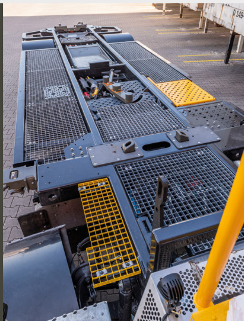
Rear guiding (air spring loaded) and jaw coupling for drawbar trailers (options).
