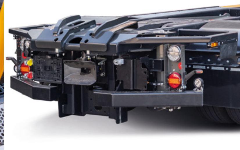
Rear guiding (air spring loaded) and jaw coupling for drawbar trailers (options).
